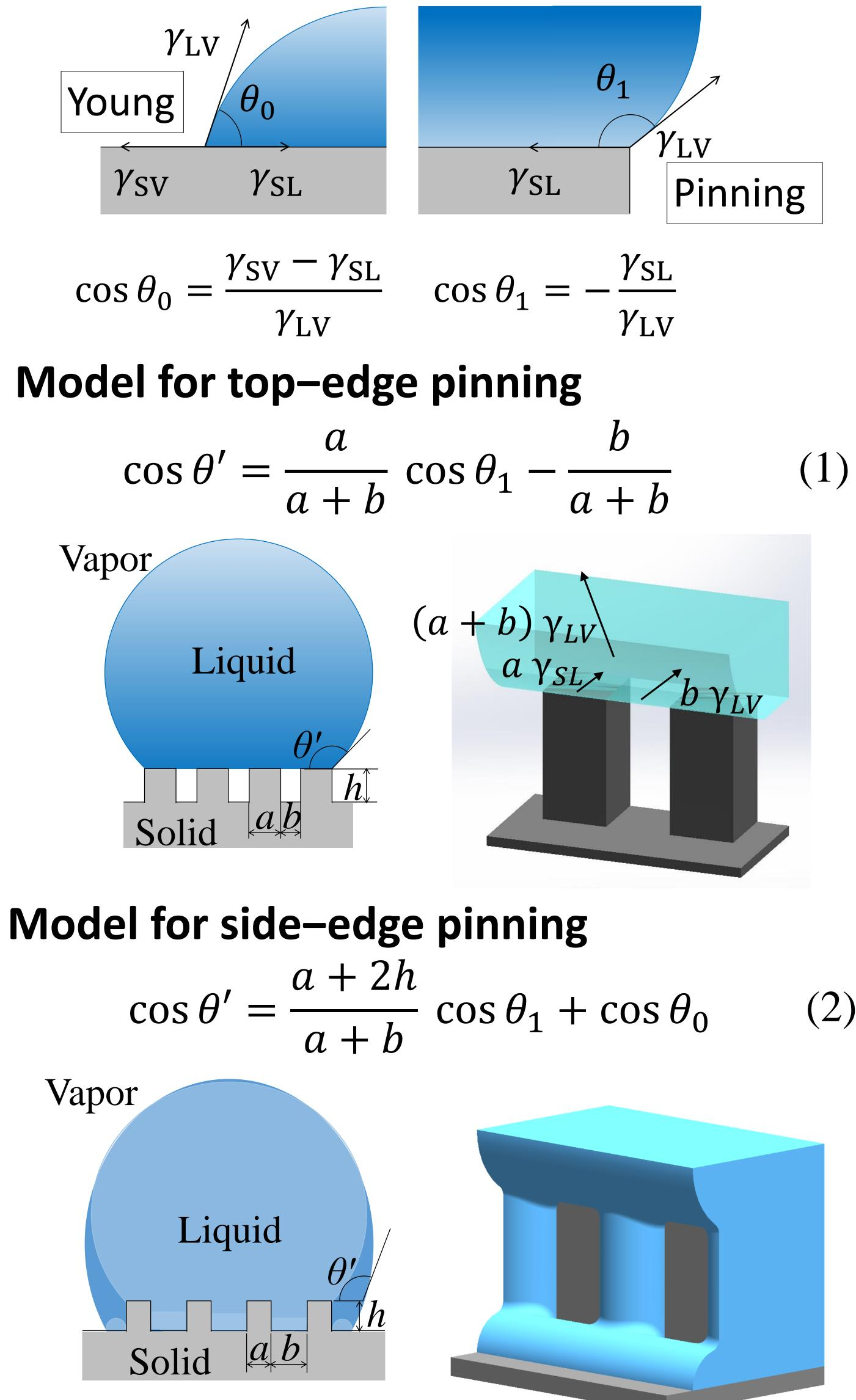
Pillar width  $a = 50 \mu m$ , groove width  $b = 100 \mu m$ ,  $\theta_0 = 114^\circ$ ,  $\theta_1 = 129.4^\circ$
